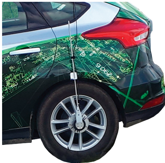
Applanix vehicle with DMI on back wheel.
