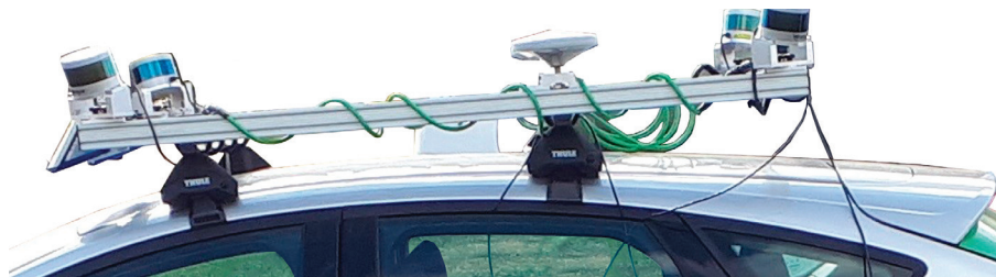
Applanix vehicle with mounted LiDAR
